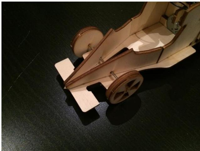
Twist the 2<sup>nd</sup> wheel onto the rod. Use the table to pressure the part in. make sure NOT TO endanger your hand by placing it on top of the rod and pushing down. Use a bit of glue if the wheels are not set on the rod.
