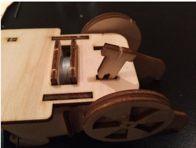
Flip the model, make sure the cog wheels are still in the right position. Then, Insert the long parts from the bottom side of the racer in order to lock the wheels in their place.
