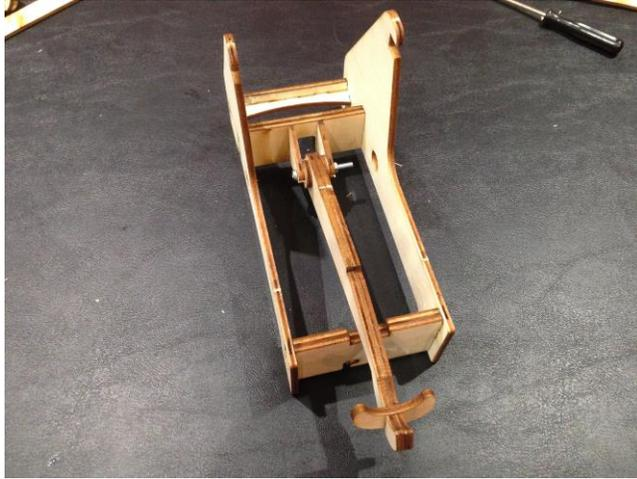
Glue the 2nd wall to its place, make sure the walls are glued well.
