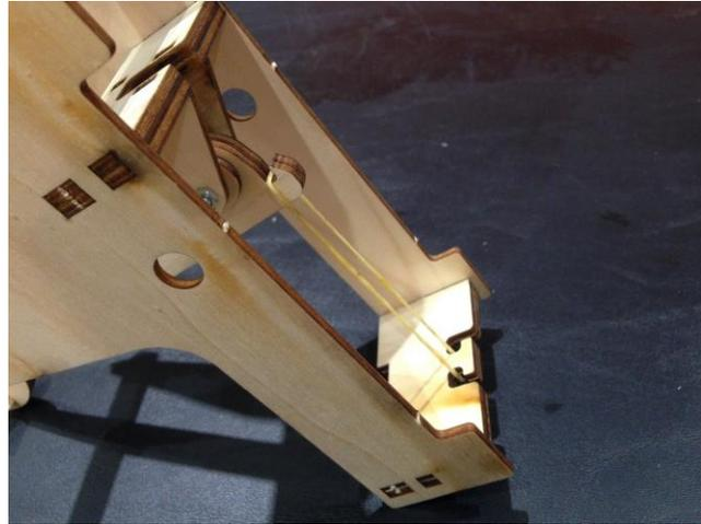
Stretch the band from the bottom part of the arm to the back part of the model.
