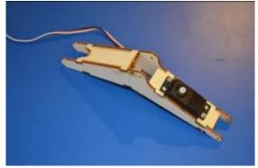
Place the servo in its place. Make sure the hinge is close to the center of the arm (red circle). Once placed correctly, secure the servo using
