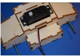
We are going to assemble the wheels onto the part shown in the picture, all the other parts should be in the plastic bag or aside.
