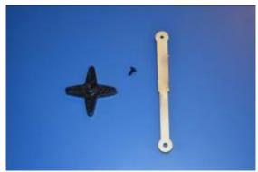
Pop out the short wooden arm as shown in the picture. Hand each student 1 bug screw and 1 servo head.
