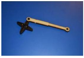
Place the servo head in its place. Make sure the bump is facing the floor. Once checked, tighten the bug screw.
