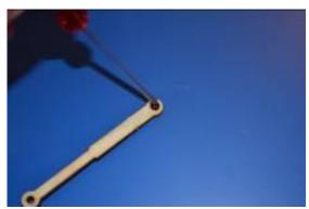
Screw just the tip of the bug screw into the small whole of the arm.
