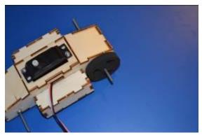
Insert one black wheel, apply a little glue on the outer side.
