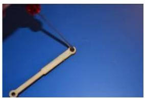
Screw just the tip of the bug screw into the small whole of the arm.
