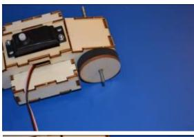
Insert 1 wooden wheel, apply a little glue on the outer side of this wheel as well.
