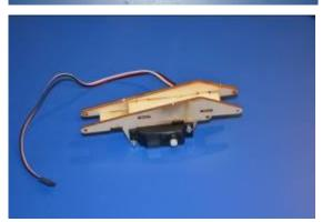
We are going to slide the servo from the outer side onto the small arm. Make sure the white hinge is close the center of the arm. Once placed correctly, secure the servo using the screws. CHECKPOINT!!! Check both servos.
