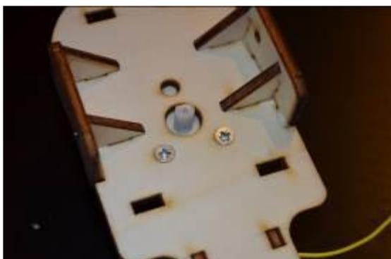
Insert the drilling screws on the other side.
