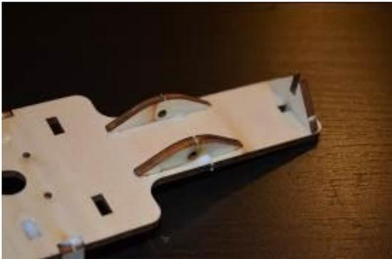
Glue the motor's base and the back triangle.
