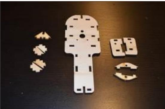
Next, disassemble and file all of the card's parts as shown in this photo. The filing is crucial. If it is not done well, the parts won't come together as they should.
