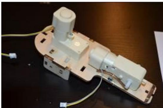
Place this motor according to the holes on the card.
