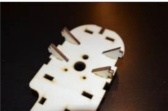
Glue the triangles to the bottom of the card (just as you've done in previous robots)
