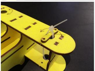
After inserting the zip tie, insert a round part into the zip tie, as shown in the picture.
