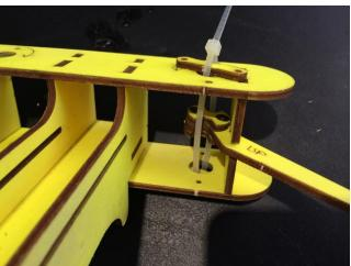
Take one arm and insert the circle on the edge into the zip tie. So the zip ties are aligned with the circle's cracks.
