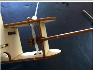
After you're done, each arm should be locked on both side with a twisted zip tie.
