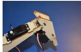
Small arm and assemble it onto the long arm, the connecting holes are the ones closest to the servo. Once checked, insert the screw and tighten with the NYLOCK. Parts should move freely.
