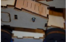
Once inserted, make sure the screw goes through the arm and out on the other side of the cabin. Place the nut on the screw, tighten, but make sure the arm can move freely
