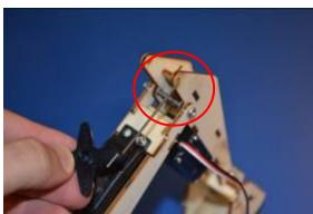
The other side of the metal bar insert into one of the rear holes of the shorter arm (red circle)
