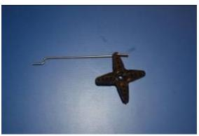
Insert the bar into one of the furthest holes on the servo head.
