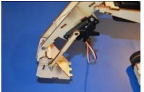
Place the servo head onto the servo, secure it in its place with a bug screw
