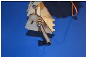
Slide the large hole onto the screw. And tighten the NYLOCK onto the screw. Make sure the parts can move freely.
