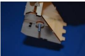
Insert the screw from inside the bucket, slide the wooden spacer on top of it from the outside.
