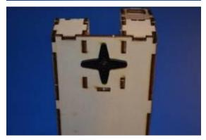
Place the servo head on the bottom side of the base. Make sure the bump on the servo head is facing the floor (so we can later connect it to a servo)
