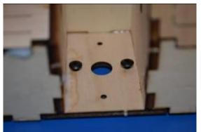
Insert the tip of the screws from the upper part (next to the driver's seat) DO NOT TIGHTEN THE SCREWS!
