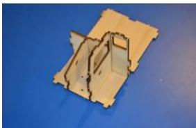
Slide the part from the top and into the base. Use glue to secure the part in its place.
