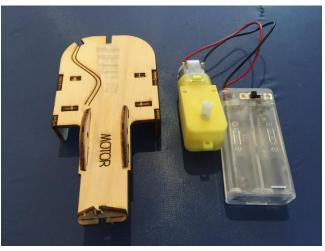
We are going to place the motor on the card. You can see the word "motor" that indicates where to place the motor.
