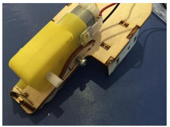
Insert the locknut from one side, through the motor, out from the other side.
