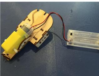
Place the motor so its bottom holes are aligned with the holes of parts marked "1"
