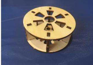
Align the holes so all the wall are inserted correctly into the large wheel.
