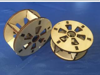
Check all the wheels, if assembled correctly, continue and assemble the  $2^{nd}$  wheel. Repeat the steps until you have 2 completed wheels.
