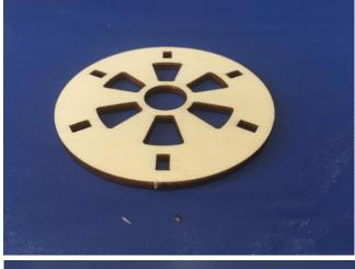
Apply glue on the top of each wall and place the large wheel on top of the walls.
