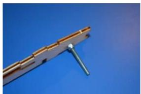
After checking both screws on the same piece are facing the same way, hand the students screwdrivers & wrenches to tighten the nylock locknuts at tight as possible. Once completed, color the model
