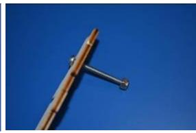
Insert the screws facing the same direction and lock with the nylock. Before tightening the locknut check the directions of the screws (red arrows)
