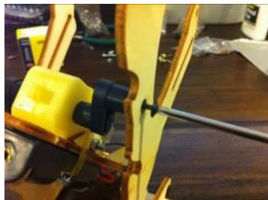
Place the leg's large hole on the crank. Notice that the front nail faces the switch. Hand each student a bug screw, screw it in and release a full turn. The foot's short part is placed under the card's front.
