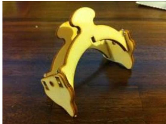
Glue ribs in their place using the walls. Notice that walls are parallel to each other as shown in this photo.
