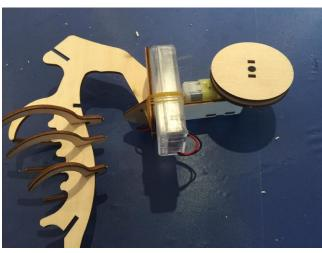
Take the wheel and place it on the motor (above the battery box). Hand the students a driller screw, and screw in into the wheel.
