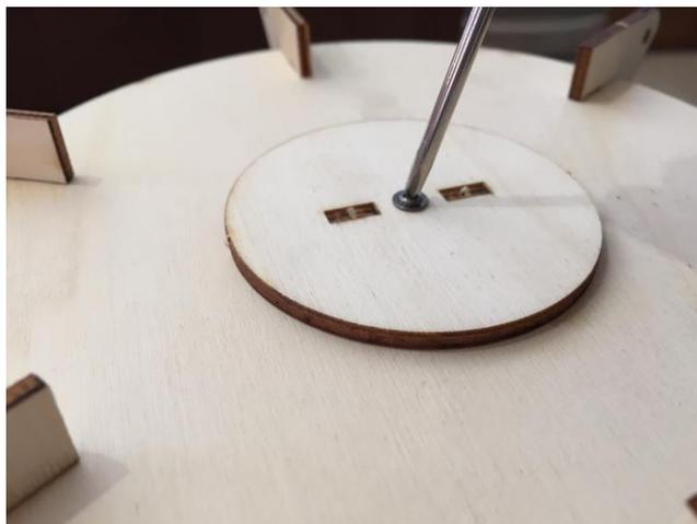
Tighten the large circle onto the motor.
