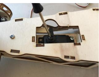
Place the servo head on top of the servo, and secure it in place using a bug screw.
