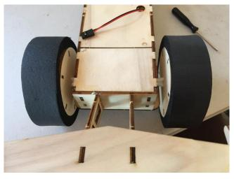
Place the tires onto the rear wheels, if need apply some glue between the tire and the wheel
