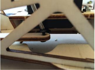
While the model stands straight, where the servo's wire is facing up, place the wooden rod on top of the servo head, screw the bug screw through the wooden part and into the servo head. DO NOT over tighten it.
