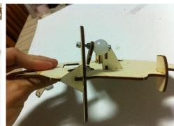
Insert the screw into the fitting hole in the eyebrow, and lock with a nylock locknut. Make sure the locknut is tightened all the way, then undo 2 full circles so that the eye can move.
