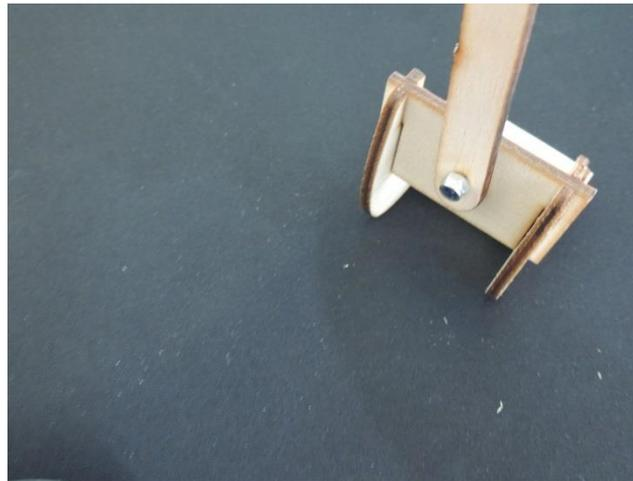
Place the long bar behind the chair, insert the screw and tighten it with the locknut.
