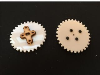
After checking the first  $\cos$  wheel, assemble the  $2^{nd}$  one.
