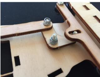
Screw the nylock onto the middle screw.
