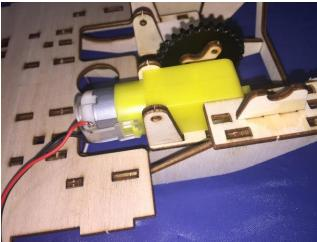
Slide the motor into its place
