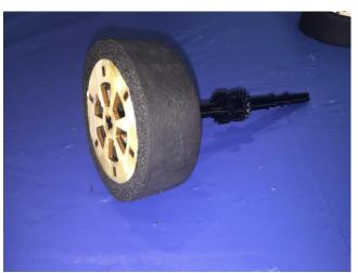
Glue one wheel, make sure the axle is inserted all the way into the wheel
