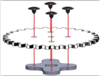
As shown in the sketch, drill the screw through the gear and into the wooden part.
