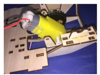
Tilt the motor so the white hinge can slide in
