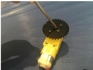
Put the gear onto the motor and screw it to its place using the bug screw
