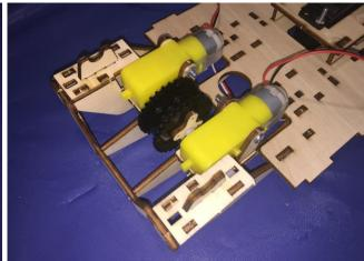
Insert the screw from the outside and place the nut from the other side.
