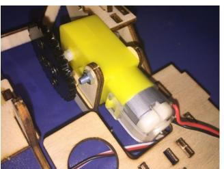
Insert the screw from the outside and place the nut from the other side.
