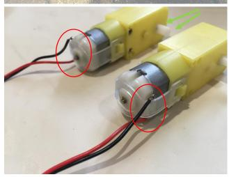
Place the motors on the table so the red wires are facing the same way, and the black wires are facing the same way.
