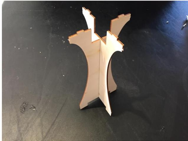
Apply glue in the cracks and slide the parts together.
