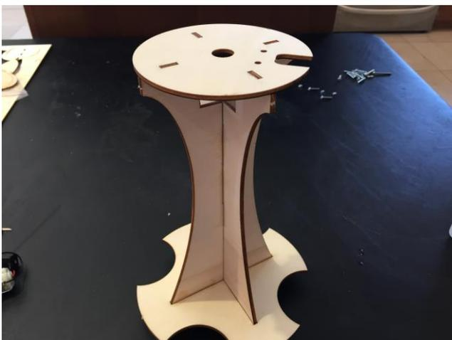
Glue the part on the top of the tower (small side)
