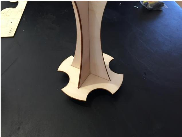
Once you slide the part all the way down to the bottom of the tower, apply glue.
