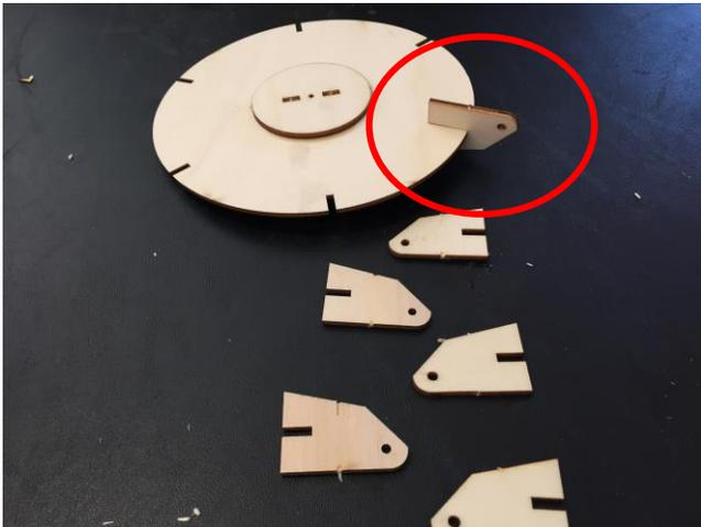
Glue the parts when the straight side is on top.
