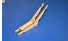
Place the parts on the table as shown in the picture. Glue the rectangular part on the top, and the other part (with the round end) to the bottom. Hold the parts together for a few minutes until the glue dries
