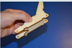
Check the bottom part. Hold the pieces together for a few minutes until the glue dries.
