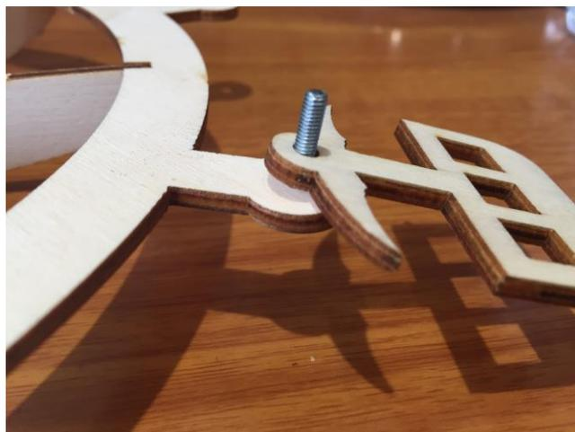
Place the cart on top of the large wheel (not under), insert the screw from the bottom part and lock it with the Nylock from the top.
