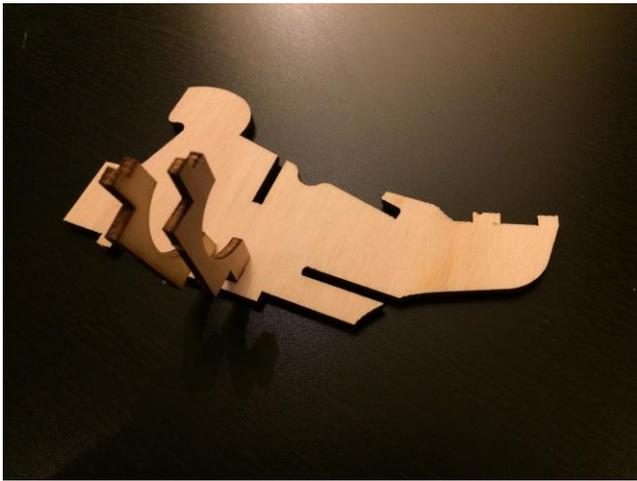
Glue the 2 gat parts when the round side is on the bottom
