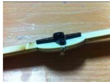
Place the servo cross exactly in the middle of the wooden circle. **The servo's part that sticks out should face upward (and not go inside the circle)**
