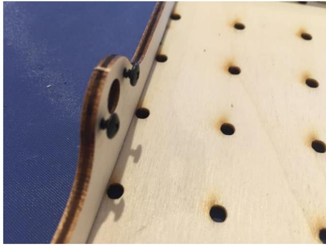
Once checked, hand the student 2 more bug screws and a round servo head. Insert both screws to the side wall of the maze. Screw the bug screws just enough to get them to the other side of the wood.
