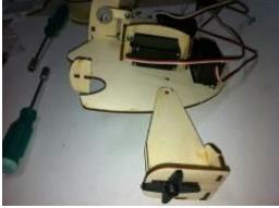
First, place neck in its place. Notice neck placement direction (back wall should be on the side farther from the eyes).
