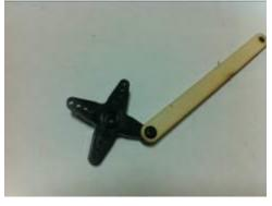
Disassemble this wooden piece. Hand each student a cross and a bug screw. Insert the bug screw into the small hole and then to the cross. Notice that the wood and the cross' sticking out side are **NOT** facing the same direction!! (Cross' sticking out side faces the table)
