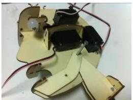
Hand each student a 30 screw. Insert the screw into the jaw, through the neck, into the face and all the way through. Let students insert the screw on their own.
