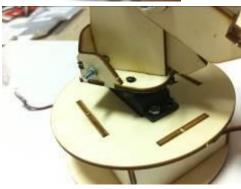
After tightening the cross to the servo, turn the neck back. This time, connect the cross's other side to the wood using the bug screw. This way, you will no longer be able to turn the neck around.
