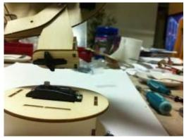
Take the assembled base, the jaw, and the face and neck. Place the cross at the neck's bottom, and connect it to the servo on the base.
