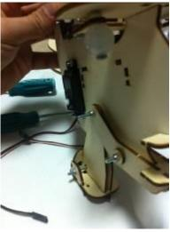
Lock the screw with a nylock locknut. Tighten the locknut all the way, then release it several full turns so that the parts will be free to move.
