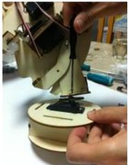
After placing the cross in its place, turn the neck so you can see the middle of the cross. As you remember, we connected the cross only to one side so we can turn the neck around and see the middle of the cross.
