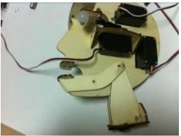
Place bottom jaw on the neck on the neck. Holes should be on top of each other. Notice the jaw's direction.
