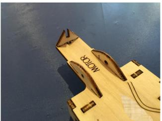
The triangle should be glued on the same side as parts #1.
