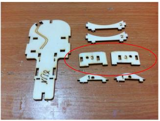
We are going to glue part #3. Please notice that on the bottom of the part we have a wide bump and a narrow bump. The bumps should fit into the card's side.
