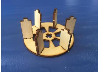
Glue the walls into the cracks on the wheel
