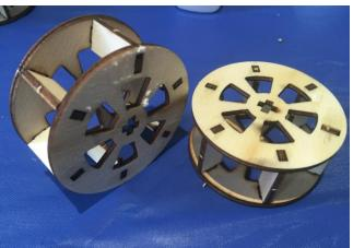
Check all the wheels, if assembled correctly, continue and assemble the 2<sup>nd</sup> wheel. Repeat the steps until you have 2 completed wheels.
