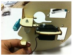
Connect servo to the face's side. Notice assembly directions.
