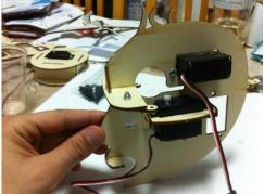
After assembling the first servo, check that all students did so correctly. Only then hand them a second servo to assemble it. Notice that the second servo is places on the face's other side (opposite of the first servo).
