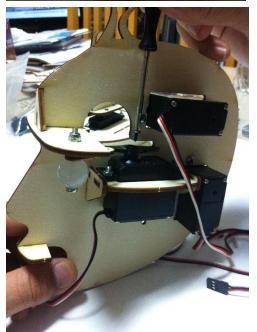
Connect a hinge (a half cross, not a full one) to the middle servo, the one under the eyebrows.
