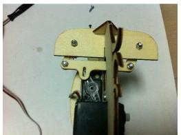
Disassemble the bridge under the eyes, and place it with the sticking out part on the left as shown in the photo. Place the bridge on the eyes' wood.
