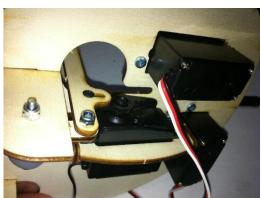
Hand students two 10 screws and 2 nylock screws. Insert the screws from under through the eye's wood into the bridge. Lock from above with a locknut. Do not tighten it all the way. Only tighten a little.
