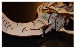
Next, connect the neck to the body. First, insert the body into the elephant (between its 2 walls).
