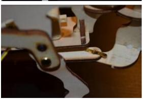
Connect the tail's bottom sticking out part to the rod coming out from the card's bottom with a paper fastener.
