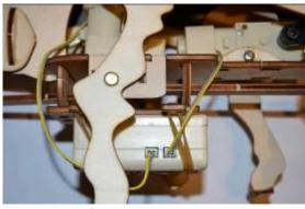
Connect the cables to their places. Connect the first motor's cable to the right, and that of the "standing" motor to the left.
