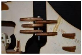
Insert the screws through all the circles' holes, so that the tail can move like a hinge next to the body.
