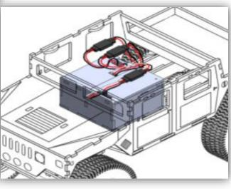
Place the smartwood control box on its mounts and connect it to the motors and servo.
