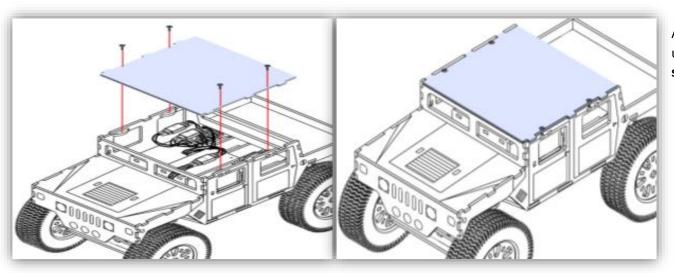
Attach the roof using four **driller** screws.
